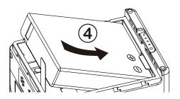
Gently pull the tape upward to remove the battery. When inserting the battery, please do not fold the tape underneath the battery.
